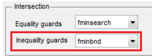
Figure 21: Dropdown menu to choose the method to be used to calculate the intersection set between sets from the flowpipe and inequality guards
